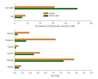
can be reduced. In particular, ash softening and corrosion affecting elements like potassium and chlorine are decreased in the press cake. In contrast, reduction of nitrogen and sulphur is only low.
