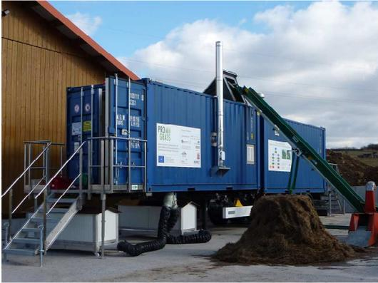
By means of a mobile PROGRASS prototype the IFBB technique is being assessed on a pilot scale, and demonstrated in 2010 and 2011 in Vogelsberg, Hesse, Germany, and in the European partner regions of Wales and Estonia. The accompanying scientific research analyses the quality of silage and fuel, the digester dynamics and the biogas yield as well as the feasibility of the technical concept in a continuously operating mode.
