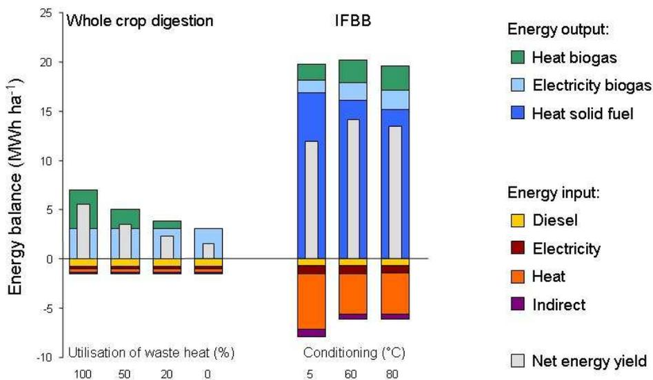
The energy inputs are higher as those of a conventional biogas plant due to meshing and drying (visualised in the lower part of the graphic), but the output of energy is three times higher (lower part of the graphic). Main product is the solid fuel which has the additional benefit of being storable and transportable.
